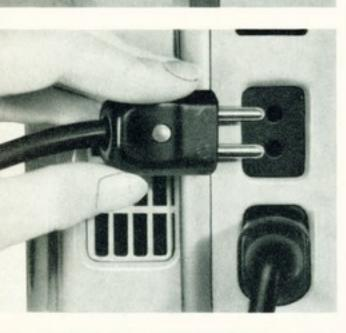
2. Use the short lead for connection to a room or table lamp which will then be switched off automatically when the projector lamp is on. (Room lamp must not exceed 70 watts).
