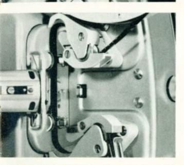
2. The film should form a loop at each end of the gate. Both loops should be evenly distributed between the loop formers and guide arms, without being in contact with either during projection.
