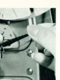
1. Open each sprocket shoe fully one at a time with the finger and insert the film on to the sprocket, making sure that the teeth are properly engaged in the film perforations.
