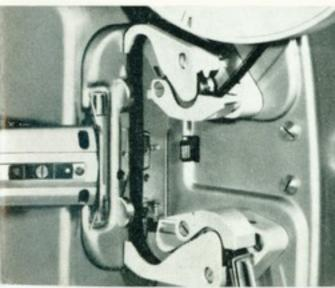
3. By depressing the upper loop-former switch (with the projector disconnected from the mains supply) both loopformers can be closed to check whether the film is correctly threaded.
