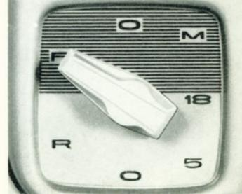
3. Turn the switch to the reverse/lamp off position.
