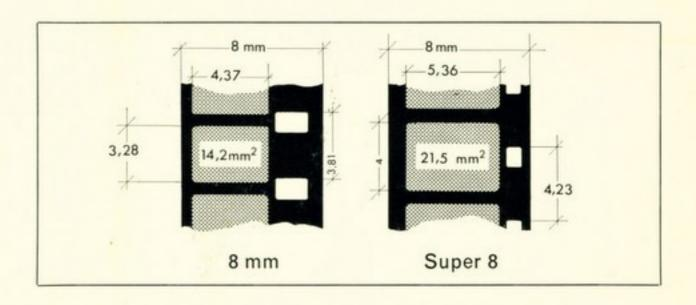
Only Super-8 film can be used in your Bolex 18-5 L Super projector. This film is supplied on spools which have a larger center hole than normal 8 mm spools.
