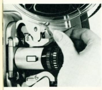
2. Insert the film leader into the slot in the upper sprocket shoe until it is taken up by the sprocket. Wait until about 1 ft. of film has passed out of the end of the film guiding channel at the rear of the projector.
