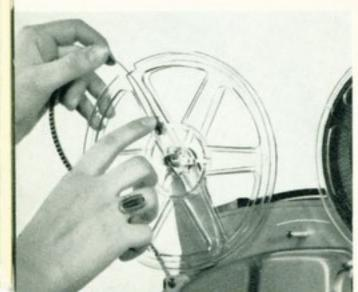
Then insert the end of the film into the slot of the takeup spool and turn it clockwise to tighten the film slightly.
