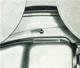
2. Pass the film over the guide post, following the line on the projector.
