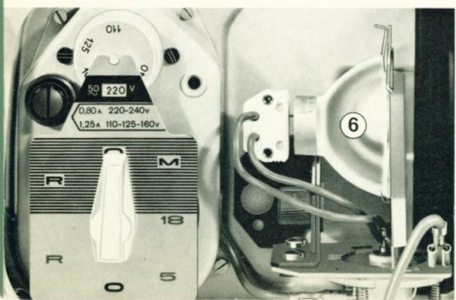
The possibility of using either the standard lamp or the 12 V/75 W halogen lamp with its incorporated cold mirror allows you complete freedom to adopt the colour temperature best suited to the different films you project.
